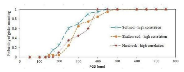
Fig. 6 Fragility curves for soft soil - highly correlated, shallow soil, and hard rock conditions based on the NZTA bridge manual requirements
