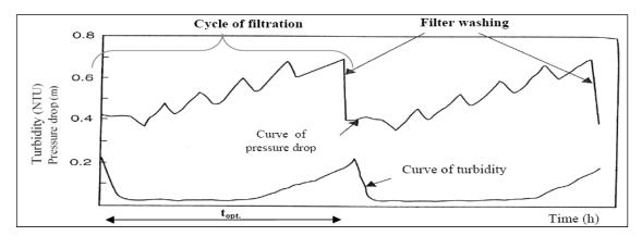
Fig. 1 A typical diagram of the dependence of filtered water turbidity and pressure losses in time – two cycles of filtration (Jusic 2012)
