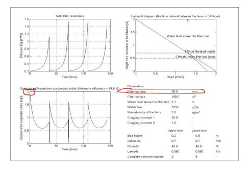
Fig. 9 Output results of simulation for input turbidity 2,0NTU – filter run time 36h (Jusic 2011)
