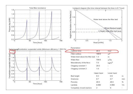
Fig. 10 Output result of simulation for input turbidity 1,8 NTU – filter run time 40h (Jusic 2011)
