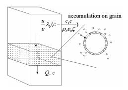
Fig. 3 Schematic impression of rapid filtration (Rietveld 2005)
