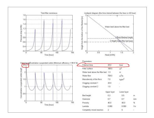
Fig. 8 Output results of simulation for input turbidity 2,5NTU – filter run time 29h (Jusic 2011)
