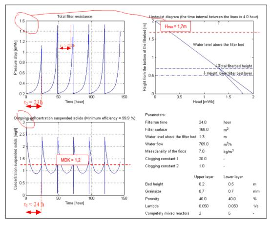
Fig. 6 Satisfactory assessment of calibration parameters - limit values set (PWTP Zenica) (Jusic 2011)
