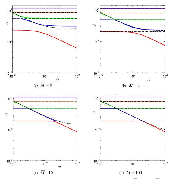
Fig. 9 Coupled natural frequencies with added mass ratio  $\overline{m}$ :  $\kappa = 100$ ; (a)  $\overline{M} = 0$ ; (b)  $\overline{M} = 1$ ; (c)  $\overline{M} = 10$ ; (d)  $\overline{M} = 100$
