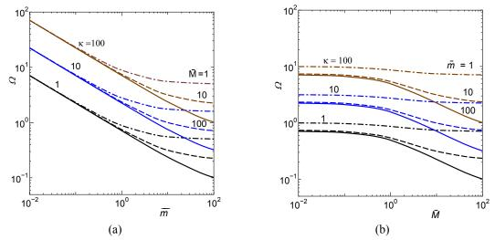
Fig. 3 Natural frequency of "spring - two masses model": ( $\kappa = 1, 10, 100$ ); (a) Variation with  $\overline{m}$ ; (b) Variation with  $\overline{M}$
