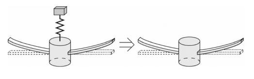
(a) (b) Fig. 5 (a) Mechanical model; (b) Elastic beam with central mass model
