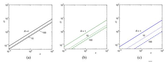
Fig. 4 Natural frequency of "spring - two masses model": Influence of spring rigidity  $\kappa$ ; (a)  $\overline{M} = 1$ ; (b)  $\overline{M} = 10$ ; (c)  $\overline{M} = 100$
