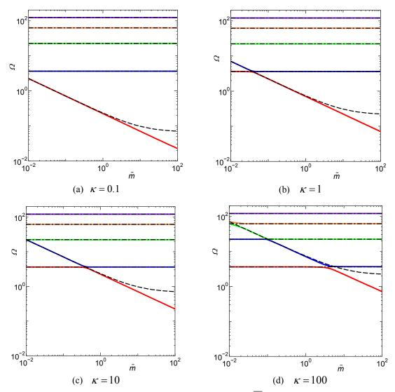
Fig. 8 Coupled natural frequencies with added mass ratio  $\overline{m}$ :  $\overline{M} = 10$ ; (a)  $\kappa = 0.1$ ; (b)  $\kappa = 1$ ; (c)  $\kappa = 10$ ; (d)  $\kappa = 100$
