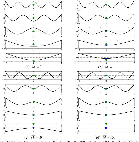
Fig. 11 Coupled vibration modes with  $\overline{M}$ :  $\overline{m} = 10$ ,  $\kappa = 100$ ; (a)  $\overline{M} = 0$ ; (b)  $\overline{M} = 1$ ; (c)  $\overline{M} = 10$ ; (d)  $\overline{M} = 100$
