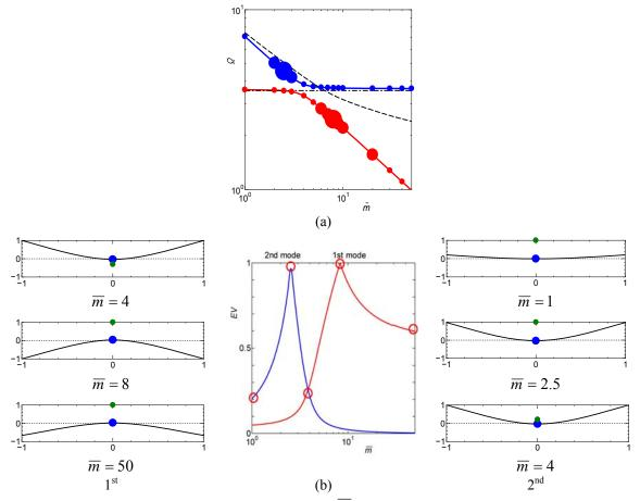
Fig. 12 Variation in evaluation value EV with  $\overline{m}$ :  $\overline{M} = 10$ ,  $\kappa = 100$ ; (a) Coupled natural frequency curves; (b) EV and vibration modes with  $\overline{m}$
