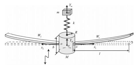
Fig. 1 Flexible spacecraft with liquid tank
