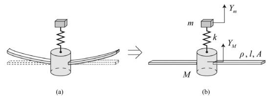
Fig. 2 (a) Mechanical model; (b) Spring-two masses model
