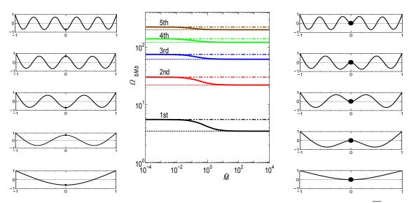
Fig. 6 Variations in natural frequencies and vibration modes of a beam with central mass M
