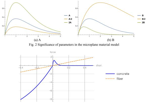
Fig. 3 Load-displacement diagram for the concrete matrix and for the fiber
