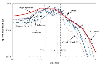
Fig. 10 Scaled earthquake spectra and target NZ design spectrum
