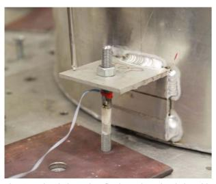
Fig. 6 Anchor bolt used to fix the tank to the shake table
