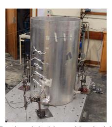
Fig. 5 Experimental aluminium model on the shake table
