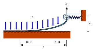
Fig. 3 Beam model used by Malhotra and Veletsos (1994a) to represent the bottom plate
