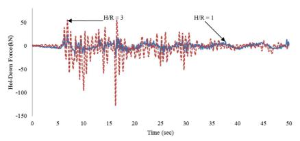
Fig. 12 Hold-down force due to the El Centro earthquake
