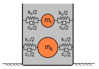
Fig. 2 Spring-mounted masses analogy for storage tanks
