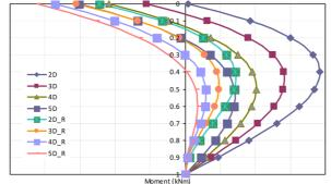
(b)Comparison of moments in front and rear pile (series configuration)
