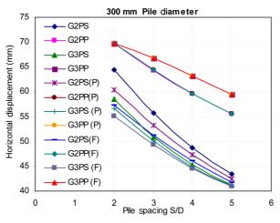
Fig. 5 Effect of pile spacing on horizonral displacement (300 mm Pile diameter)
