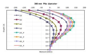
Fig. 6 Variation of moment along depth of piles in group of two piles
