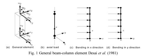
v, axial displacement w, and rotation about three axes (Fig. 1).
