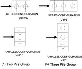
Fig. 3 Different configurations considered in the study
