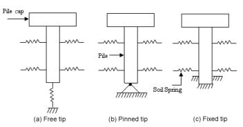
Fig. 4 Different end conditions assumed to prevail at the pile tip
