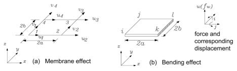
Fig. 2 A schematic of general plate element Zienkiewicz (1977)
