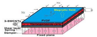
Fig. 1 Schematic of viscoelastic piezoelectric composite sandwich structures on viscoelastic foundation
