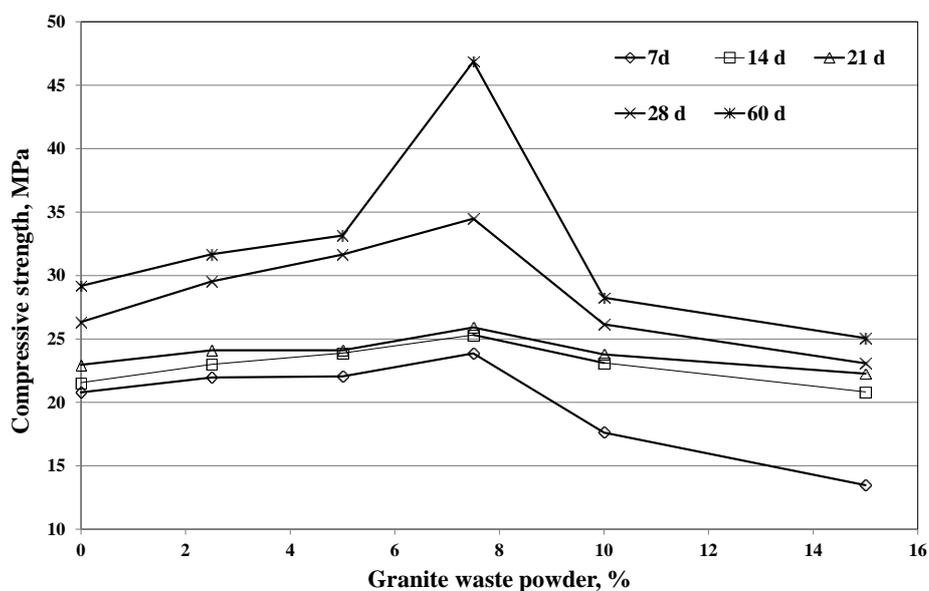
Fig. 4 Compressive strength of alkali activated mortars enhanced with various ratios of granite powder and having 5% calcium hydroxide
