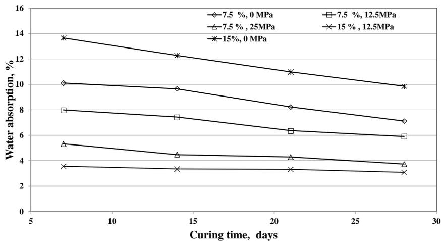
Fig. 7 Water absorption of alkali activated mortars having various ratios of granite powder, pressed at various pressing pressure
