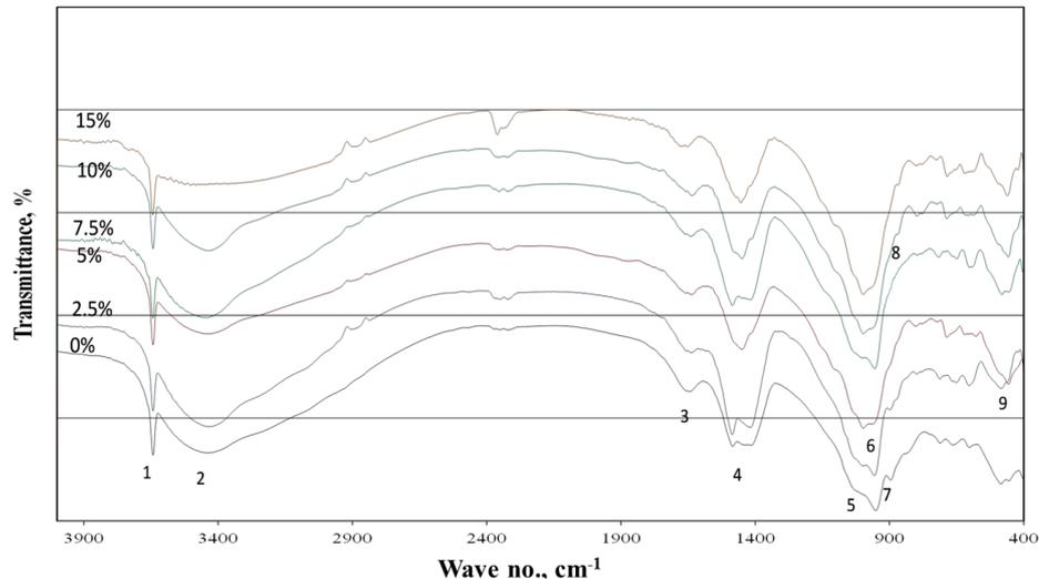
Fig. 2 FTIR spectra of 28 days alkali activated mortars having various ratios of granite powder (1,2: Stretching vibration of O-H bond, 3: Bending vibration of (HOH), 4: Stretching vibration of CO<sub>2</sub>, 5: Asymmetric stretching vibration (Si-O-Si), 6: Asymmetric stretching vibration (T-O-Si), 7: Si-O Stretching, OH bending (Si-OH), 8: out of plane bending vibration of CO<sub>2</sub>, 9: Bending vibration (Si-O-Si and O-Si-O))
