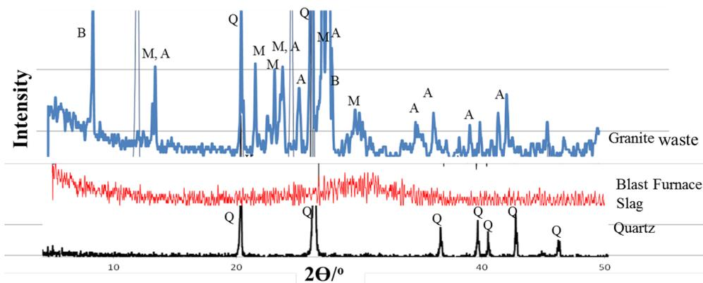
Fig. 1 Xray diffraction pattern of the starting raw materials (Q: Quartz, M-Microcline, B=Biotite, A-Albite)
