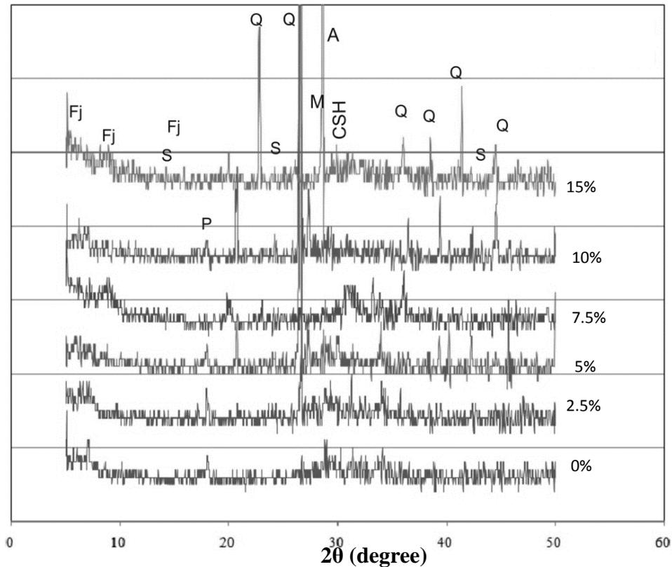
Fig. 3 XRD pattern of 28 days alkali activated mortars enhanced with various ratios of granite powder (Q: Quartz, Fj: Fanjasite, A: Albite, C: Calcite, S: Sodalite, P: Portlandite, CSH: Calcium silicate hydrate, M: Microcline)
