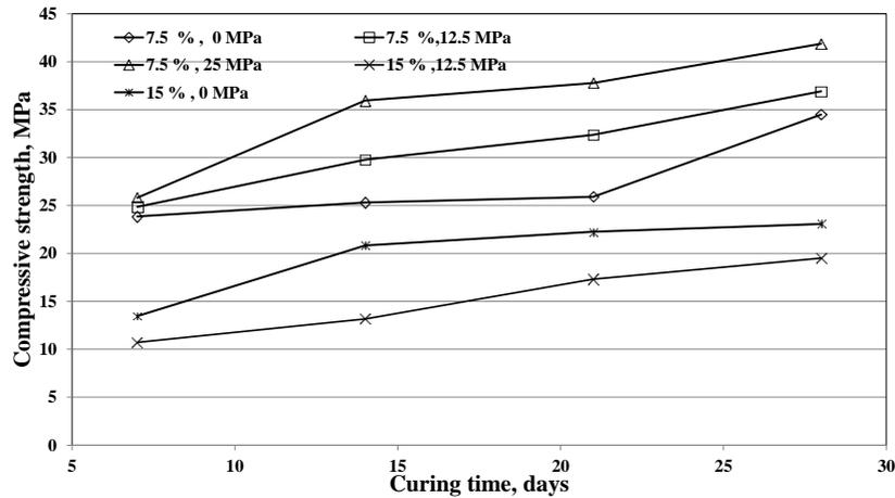
Fig. 6 Compressive strength of alkali activated mortars having various ratios of granite powder, pressed at various pressing pressure
