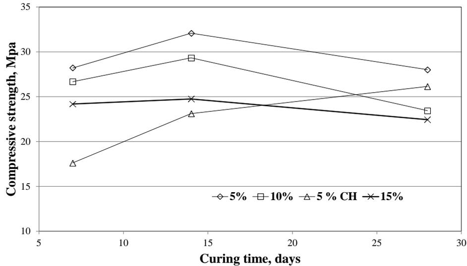
Fig. 5 Compressive strength of alkali activated mortars enhanced with various ratios of granite powder without calcium hydroxide and compared with mix having 5% calcium hydroxide
