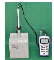
(b) Depth magnetic probe in SFRC sample
