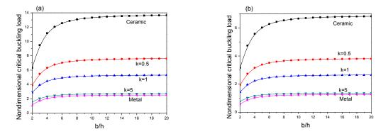
(a) Plate subjected to uniaxial compressive load (b) Plate subjected to biaxial compressive load  $(\gamma = 0)$   $(\gamma = 1)$
