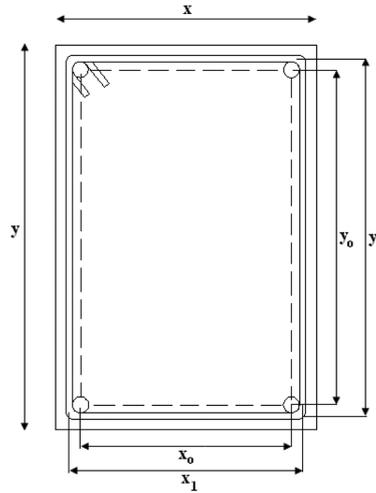
Fig. 1 The cross section of a rectangular reinforced concrete beam
