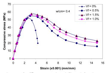
Fig. 5 Typical stress-strain curve for SF concrete and steel fiber reinforced concrete (w/cm = 0.40, SF content = 10%)
