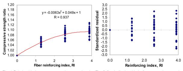
Fig. 1 Relationship between compressive strength ratio Fig. 2 Standardized residuals for compressive strength  $(f_{cf} / f_c)$  and fiber reinforcing index (RI)
