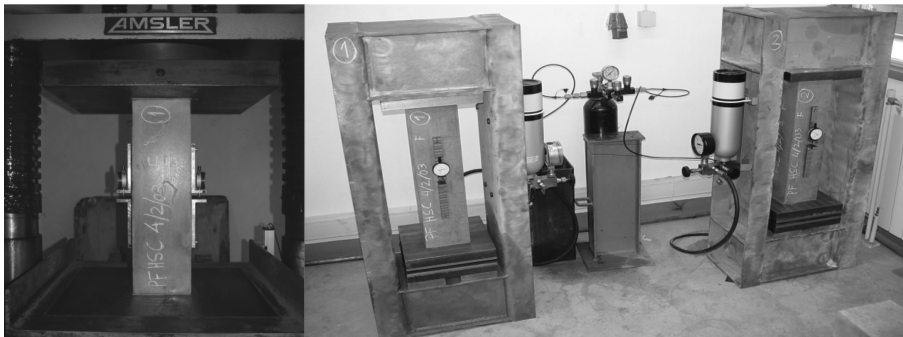
Fig. 6 (a) Equipment for evaluating compressive strength and Young modulus and (b) creep tests equipment
