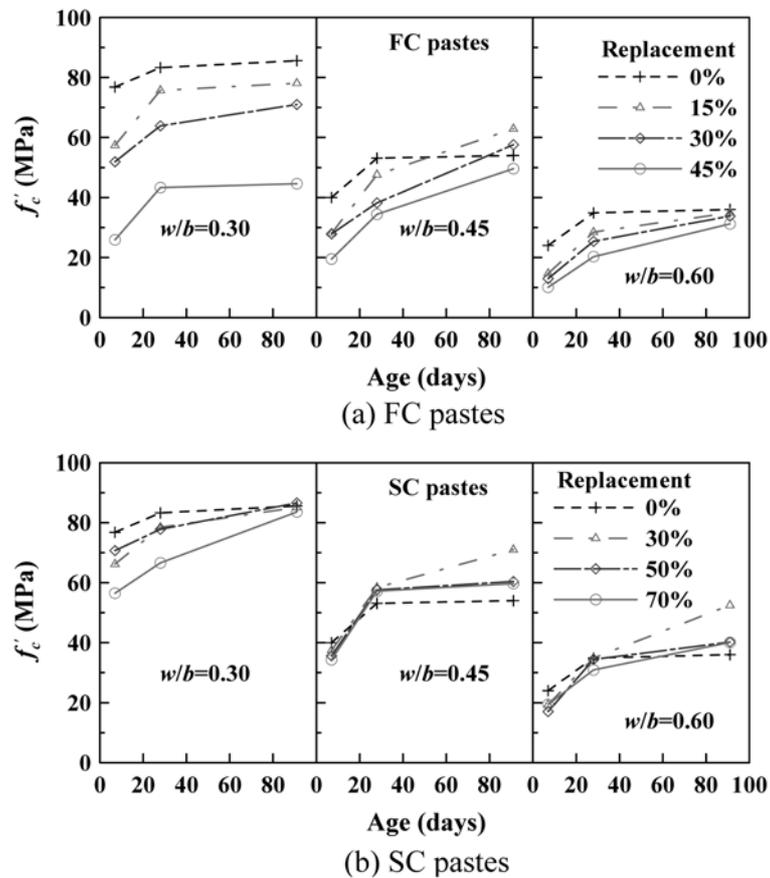
Fig. 1 Strength versus age for pastes at different  $w/b$  ratios
