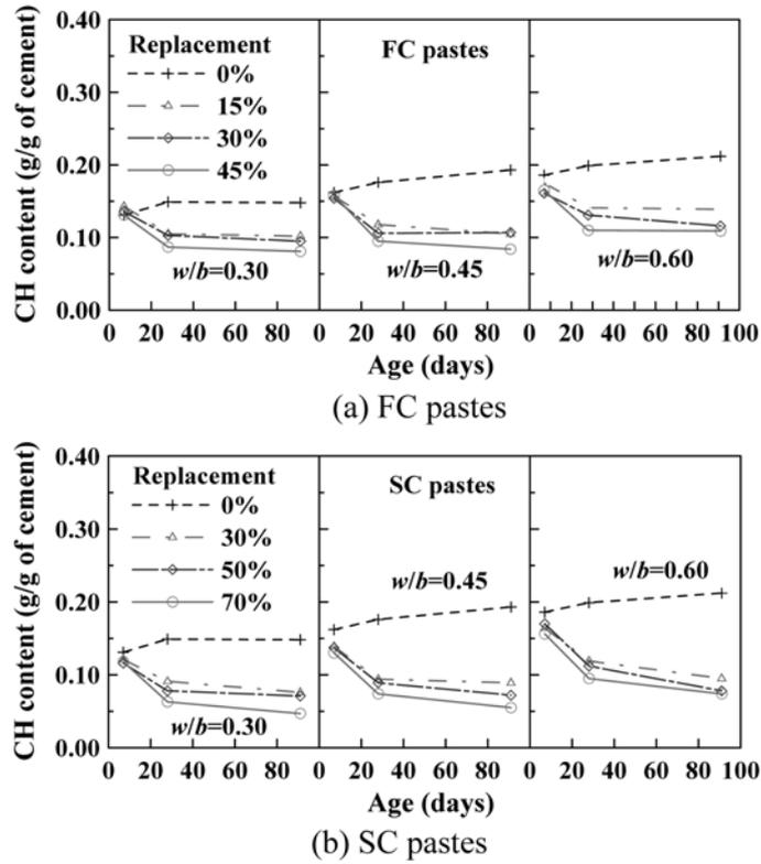
Fig. 3  $\text{Ca}(\text{OH})_2$  content versus age for pastes at different  $w/b$  ratios
