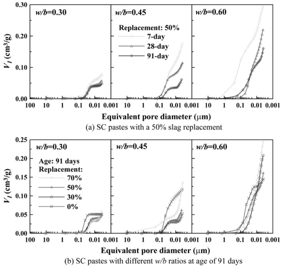
Fig. 8 Cumulative intruded pore volume versus equivalent pore diameter for SC pastes
