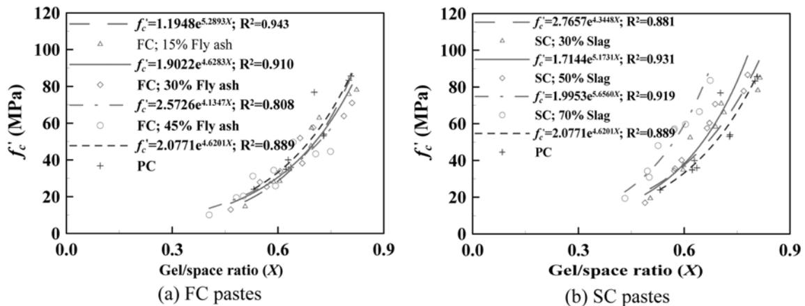
Fig. 10 Relationship between compressive strength and gel/space ratio of pastes
