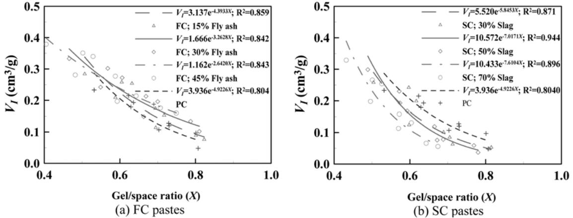
Fig. 12 Relationship between intruded pore volume and gel/space ratio of pastes
