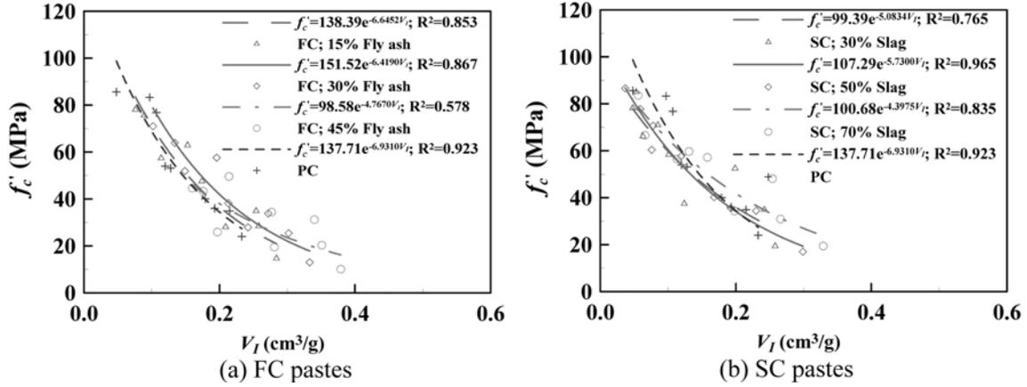
Fig. 11 Relationship between compressive strength and intruded pore volume of pastes
