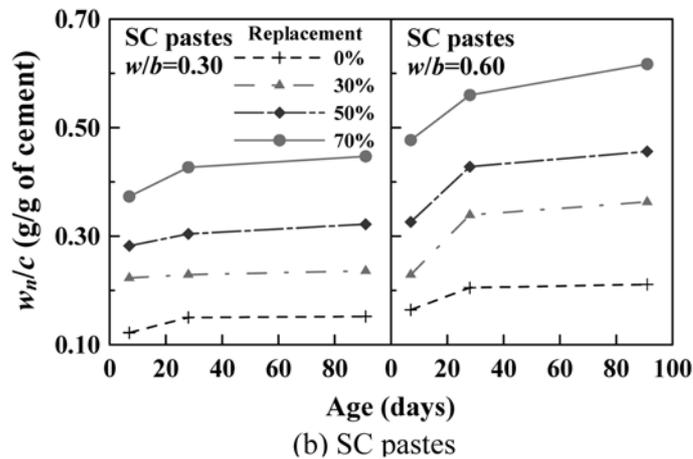
Fig. 2 Non-evaporable water content versus age for pastes
