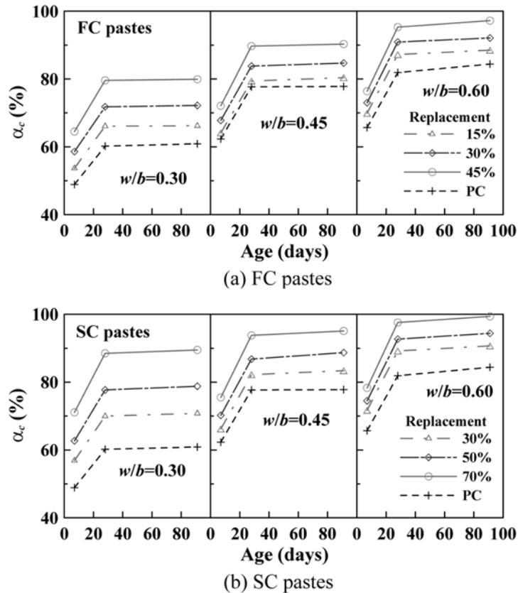
Fig. 9 Degree of cement hydration versus age for pastes at different  $w/b$  ratios
