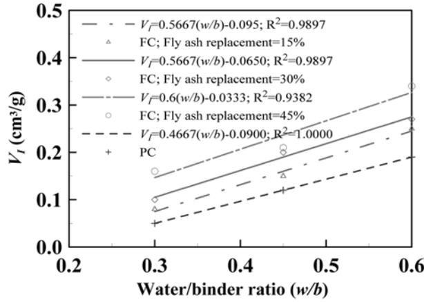
Fig. 6 Correlation between intruded pore volume and  $w/b$  for FC pastes at 91 days
