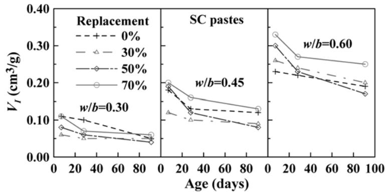
Fig. 7 Intruded pore volume versus age for SC pastes at different  $w/b$  ratios
