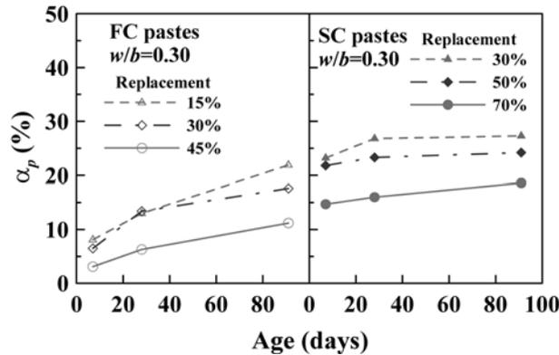
Fig. 4 Degree of pozzolanic reaction versus age for pastes with  $w/b$  ratio=0.30
