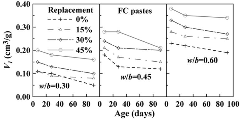
Fig. 5 Intruded pore volume versus age for FC pastes at different  $w/b$  ratios
