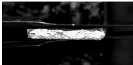
Immersion duration – 8640 hours (12 months); lateral specimen view c) concentration of \text{Na}_2\text{SO}_4 in the solution – 10%
