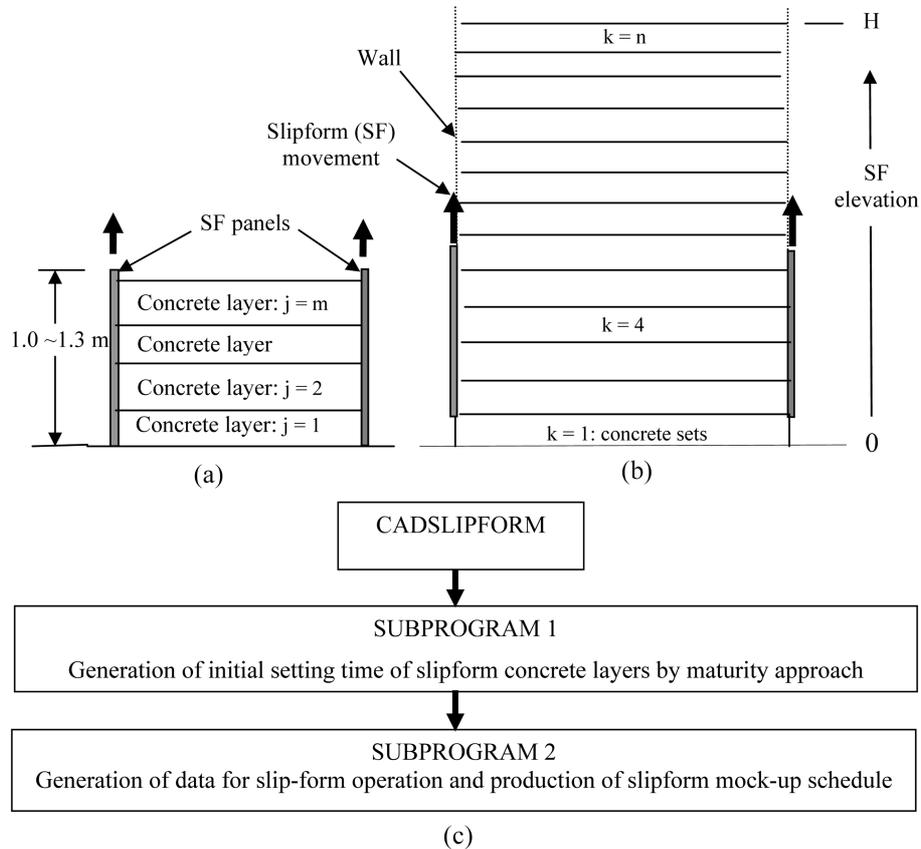
Fig. 2 (a) Typical slipform with concrete layers, (b) Slipforming operation in a wall, (c) CADSLIPFORM Subprograms
