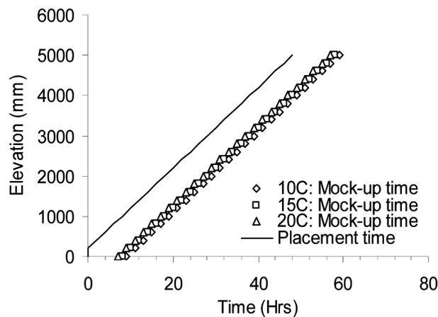
Fig. 15 Effect of variable constant temperature (in all layers) on mock-up time
