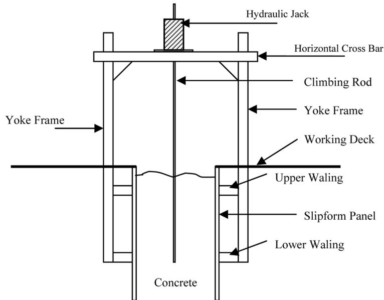
Fig. 1 Schematic diagram of a typical slipform System (Fossa 2001)
