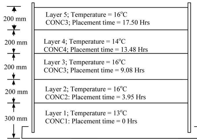
Fig. 10 Layer arrangement of slipform in the wall
