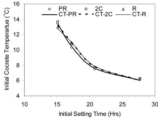
Fig. 6 Comparison of actual and predicted initial setting times
