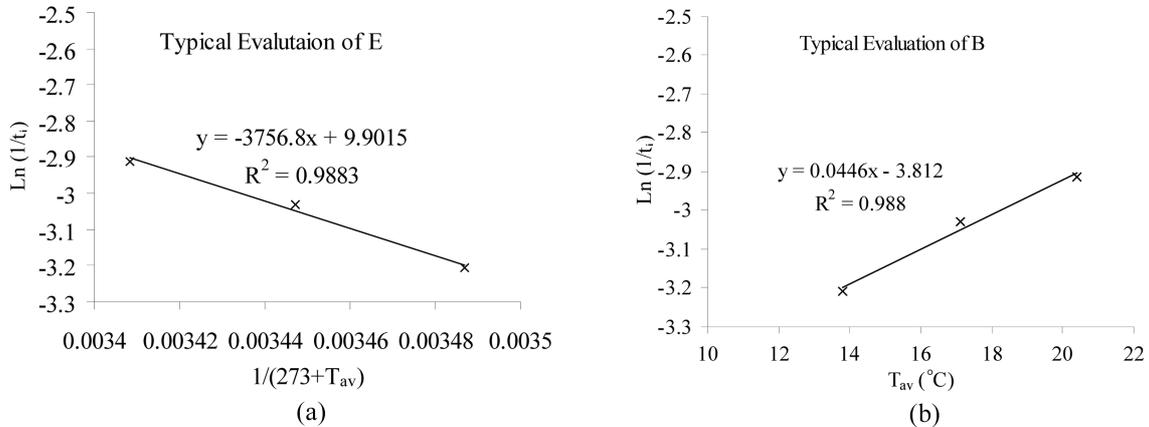
Fig. 4 (a) Arrhenius plot for the prediction of  $Q$  and  $E$ , (b) Procedure for the prediction of  $B$
