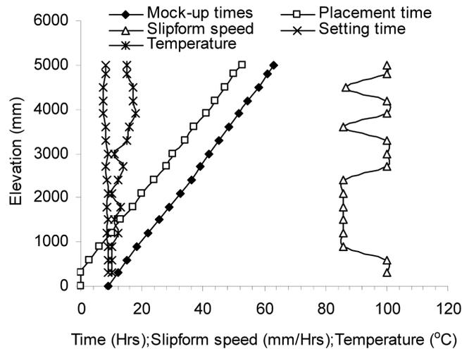
Fig. 16 Effect of variable concrete temperature in concrete layers and slipform speed on mock-up time
