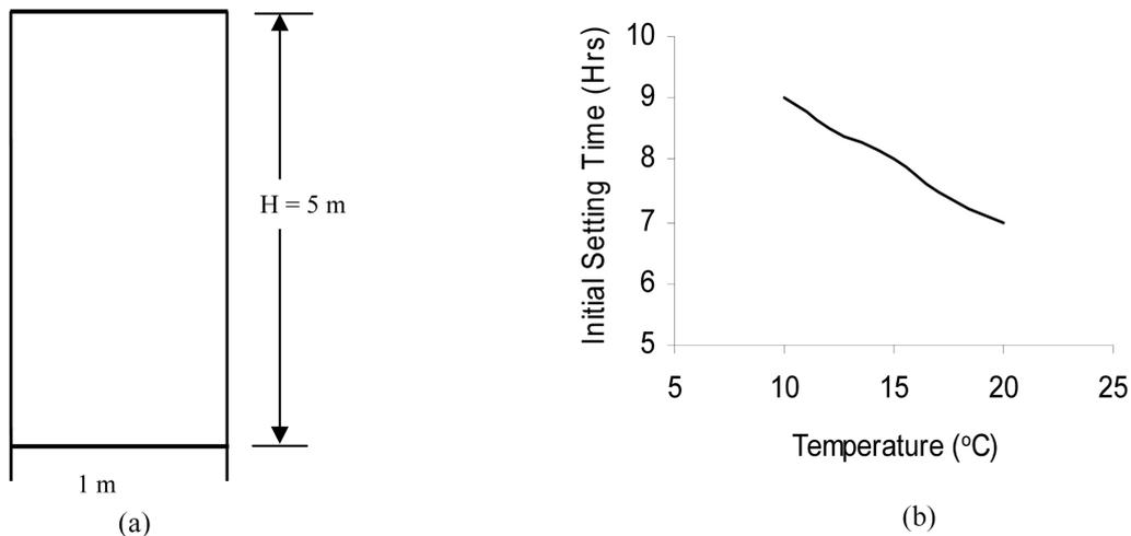
Fig. 13 (a) Wall element for parametric study, (b) Initial setting time by SUBPROGRAM 1
