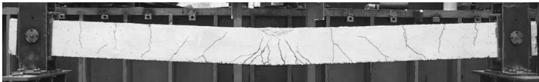
(b) Experimental crack pattern at end of test
