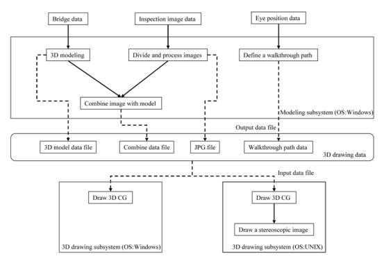
Fig. 1 VR/3DCG system components
