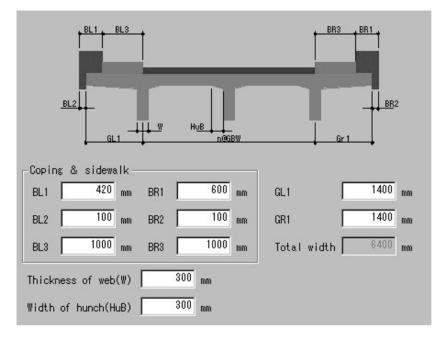
Fig. 2 Screen for defining bridge superstructure cross section
