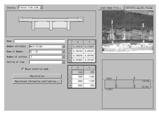
Fig. 3 Sample screen for combining the image with the model
