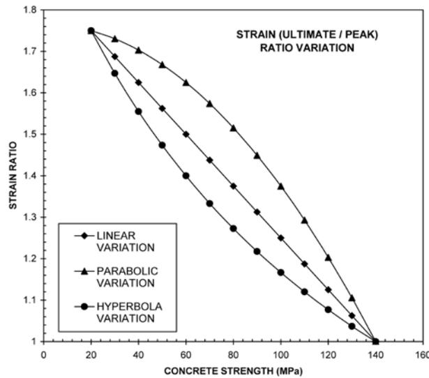
Fig. 4 Variations of strain ratio used in analysis
