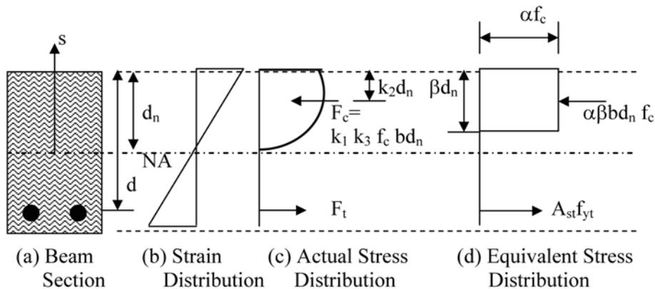
Fig. 1 Concept of equivalent rectangular stress block
