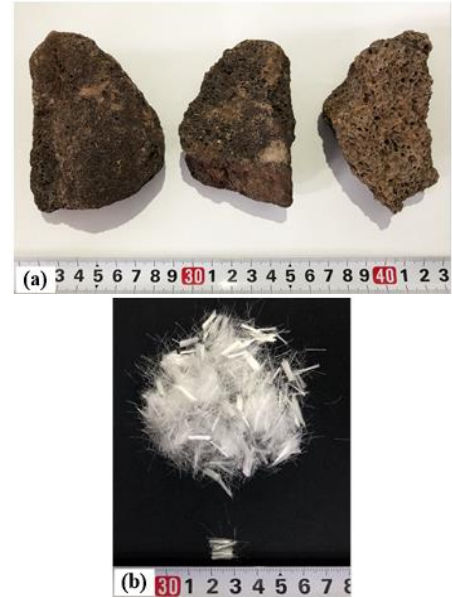
Fig. 1 Appearance of the materials used (a) Natural Cinder aggregate (b) Polypropylene Fibers
