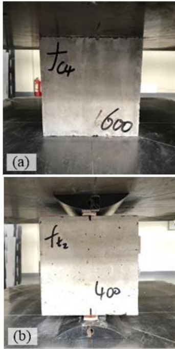
Fig. 2 Cubic concrete strength test(a)Axial compressive strength test, (b) Tensile Splitting tensile strength test
