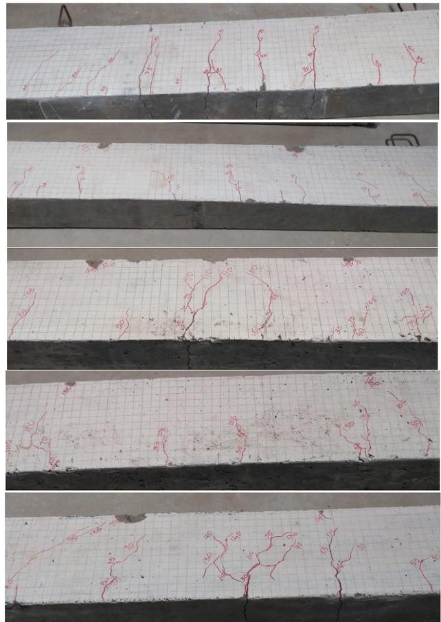
Fig. 8 Typical failure pattern of concrete castellated beams (CB, CESB, CESB- H1, CESB- H2 and CESB- H3)
