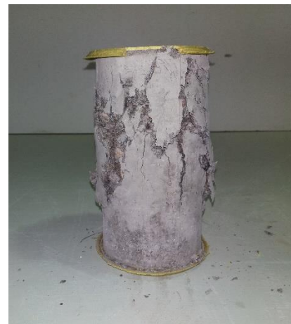
Fig. 5 Failure type in compression
