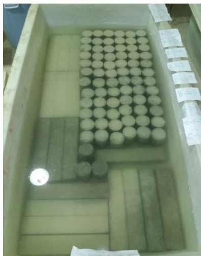
Fig. 3 Placing the specimens under the 100% relative humidity
