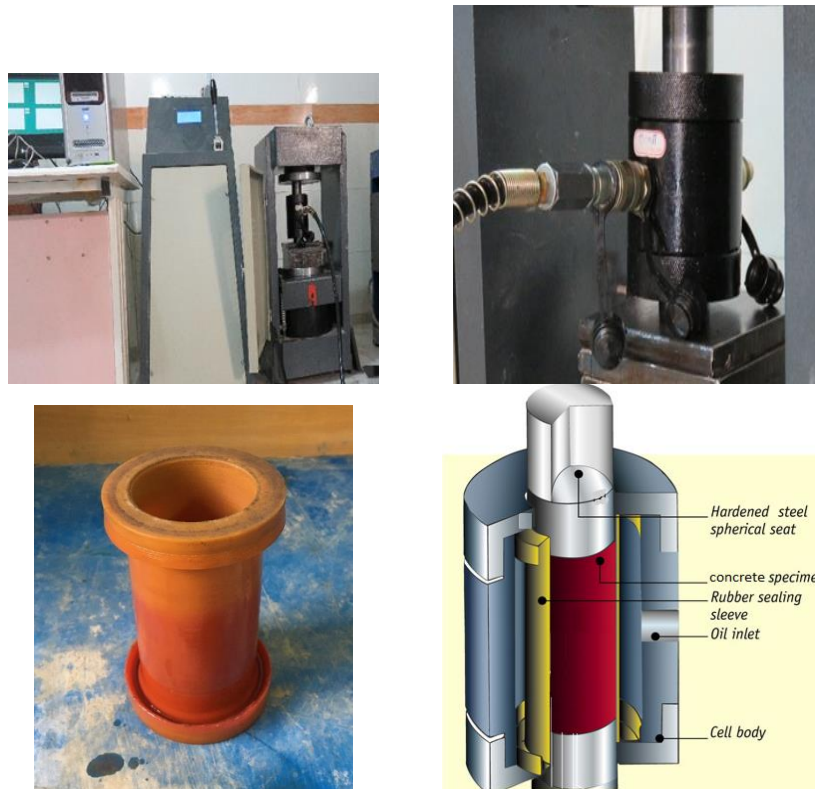
Fig. 2 General view of the 3000-kN capacity testing machine, the rubber bladder and the Hoek cell installed on this machine to apply confining pressure
