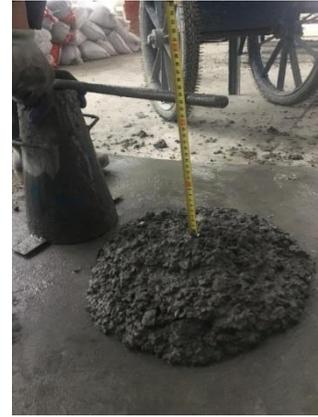
Fig. 1 The slump test of fresh concrete
