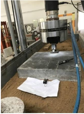
Fig. 19 Loading form of foundation bearing displacement loading control method
