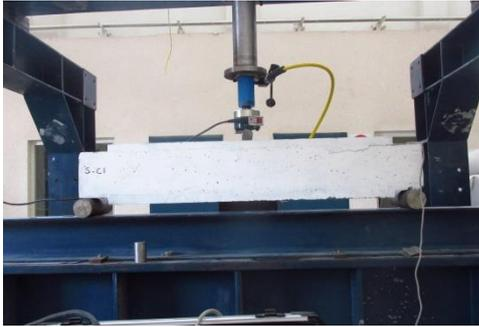
Fig. 6 The Loading setup
