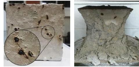
Fig. 15 The effect of temperature increase on a specimen containing forta-ferro fibers at 400°C; (a) surface of specimen and (b) specimen after compressive strength test
