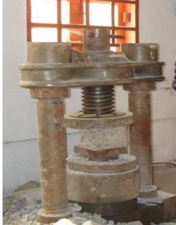
(b) Compressive strength test set up
