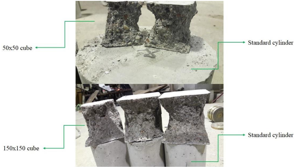
Fig. 10 Pattern of compressive failure in SCLC 50×50×50 and 150×150×150 mm 3 cubes
