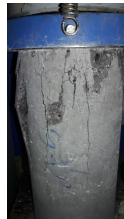
Fig. 9 Axial splitting cracks in a compressive test of cylindrical SCLC specimen
