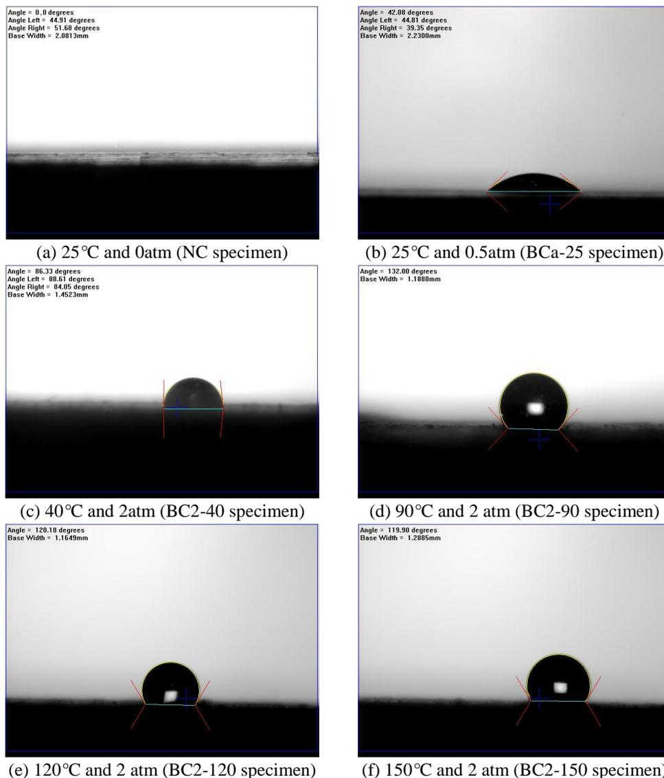
Fig. 2 Static water contact angle images of the concrete samples with various carbonation treatments
