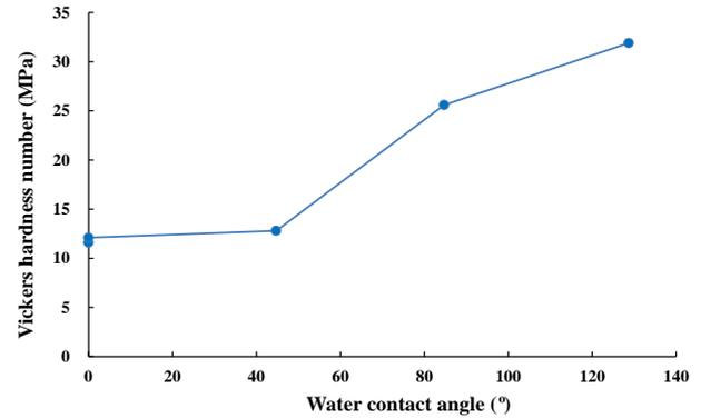
Fig. 10 Relationship between static water contact angle and microhardness of concrete
