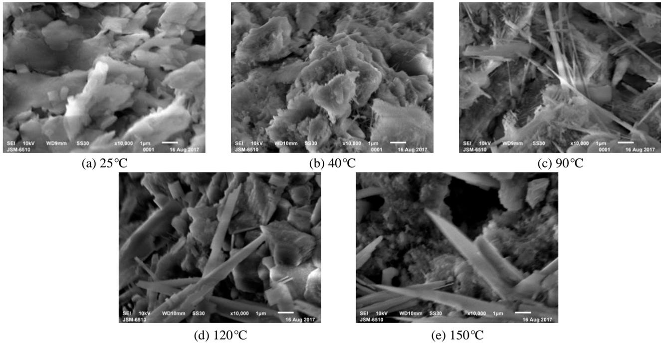
Fig. 5 SEM images of the carbonated specimens at various temperatures
