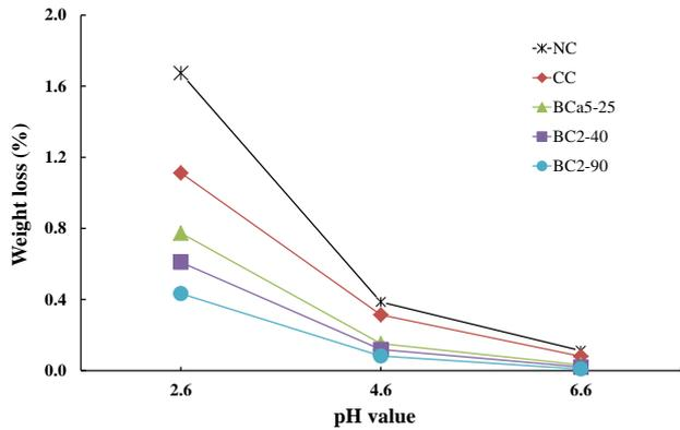
Fig. 8 Weight loss of concrete under various pH value of solution
