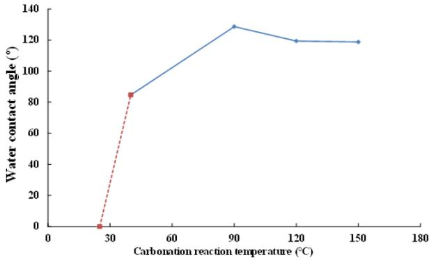
Fig. 1 Static water contact angle values of concrete surface at various temperatures
