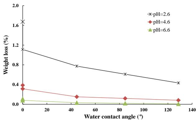
Fig. 9 Relationship between static water contact angle and Weight loss of concrete
