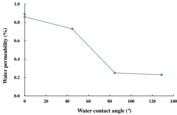
Fig. 6 Relationship between static water contact angle and water permeability of concrete
