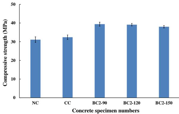
Fig. 3 Compressive strength of concrete cylinders with various carbonation treatments
