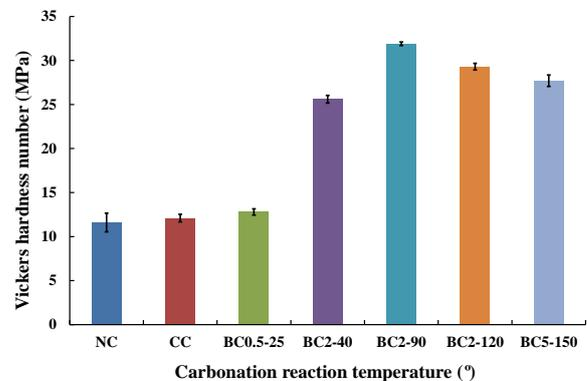
Fig. 4 Microhardness of concrete obtained at different carbonation reaction temperatures with and without sodium stearate
