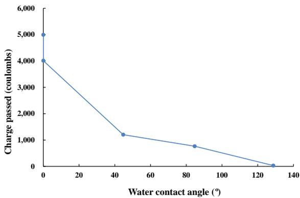
Fig. 7 Relationship between static water contact angle and charge passed of concrete
