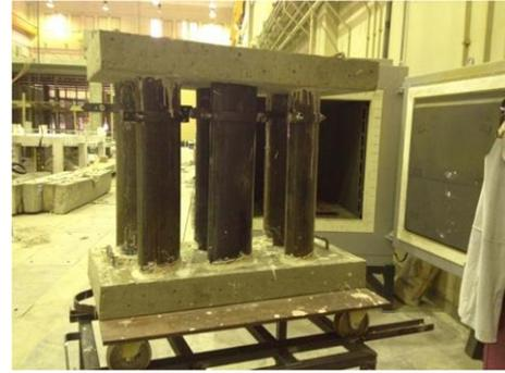
Fig. 4 Column specimens after taking out from the oven (Abbas *et al.* 2017)
