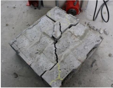
Fig. 13 Typical failure of the specimen
