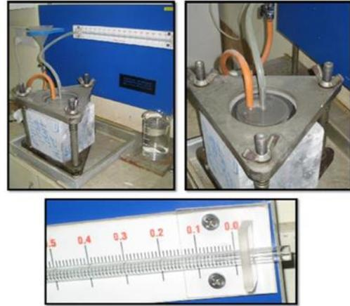
Fig. 1 Initial surface absorption test
