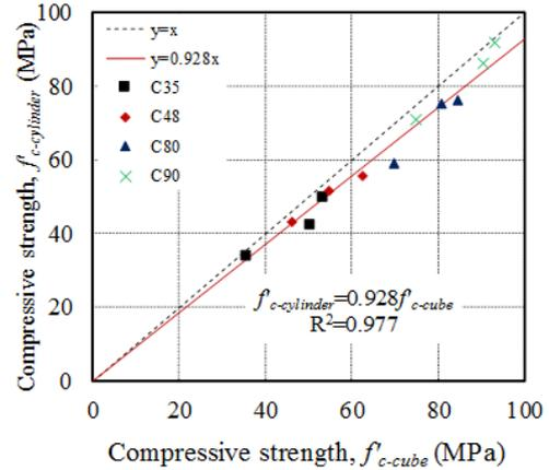
Fig. 5 Relationship between the cubic and cylindrical compressive strength of SCCs
