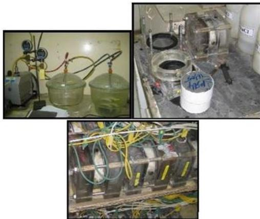
Fig. 3 Rapid chloride permeability test
