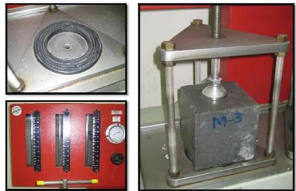
Fig. 2 Water permeability test
