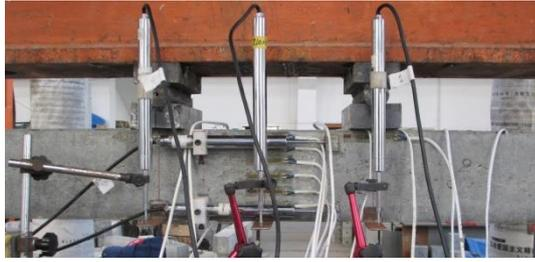
Fig. 6 Loading and measuring arrangement of test beam
