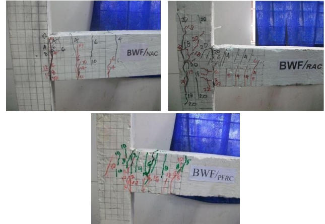
Fig. 8 Failure modes of BWF specimens
