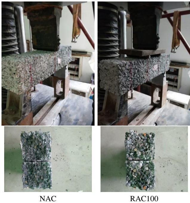
Fig. 7 Failure of pervious concrete specimen under splitting tensile test
