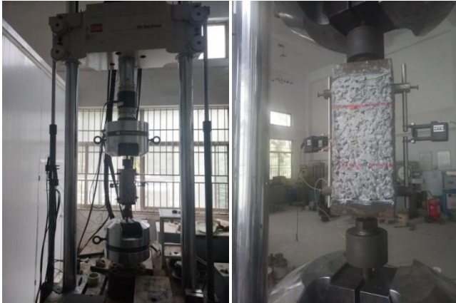
Fig. 9 Direct tensile test of pervious concrete with MTS test machine
