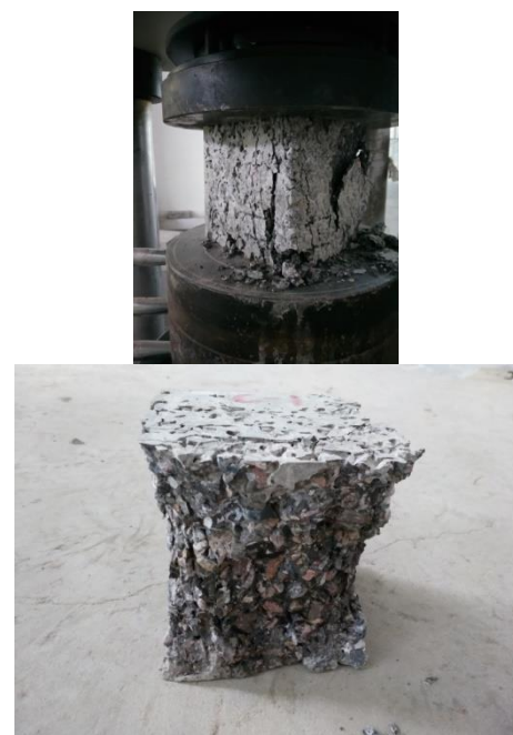
Fig. 3 Failure of pervious concrete specimen under uniaxial compression
