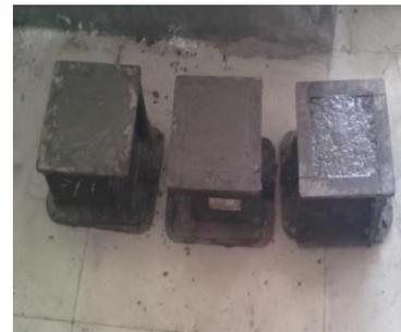
Fig. 3 Geopolymer concrete cube moulds
