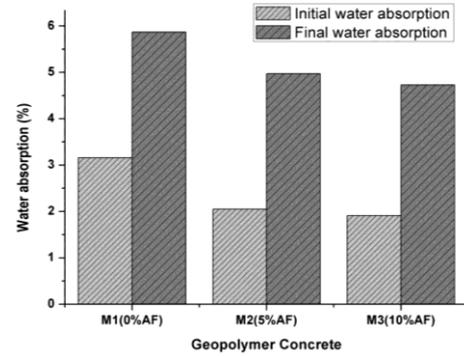
Fig. 9 Effect of Alccofine contents on initial and final water absorption
