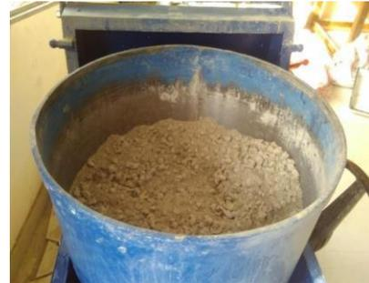
Fig. 2 Mixing of materials in pan mixer
