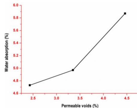
Fig. 11 The relationship between permeable voids and water absorption
