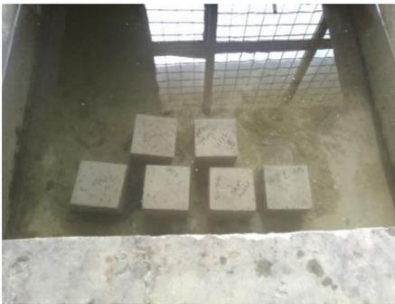
Fig. 5 Water absorption test
