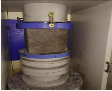
Fig. 4 Compressive strength testing
