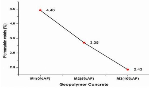
Fig. 7 Effect of Alccofine contents on permeable voids
