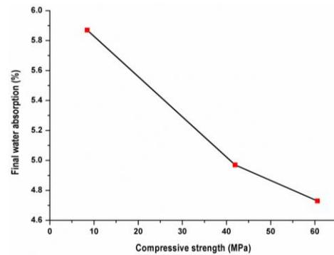
Fig. 10 Variation of final water absorption with compressive strength
