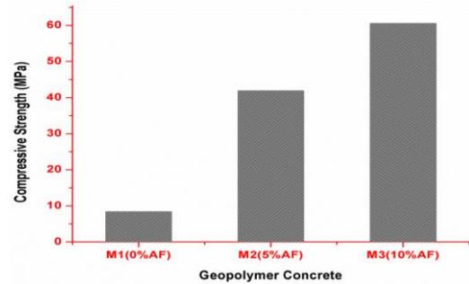
Fig. 6 Effect of Alccofine contents on compressive strength
