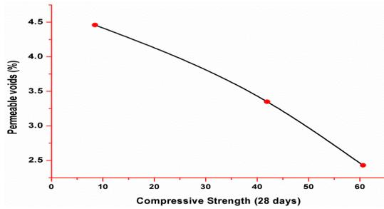
Fig. 8 Variation of permeable voids with compressive strength
