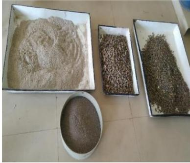
(a) Coarse and fine aggregates with fly ash
