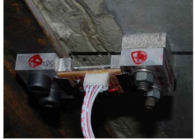
(b) Installed relative displacement sensor
