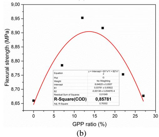
Fig. 10 Variation of (a) compressive and (b) flexural strengths with respect to GPP replacement at the age of 28 d
