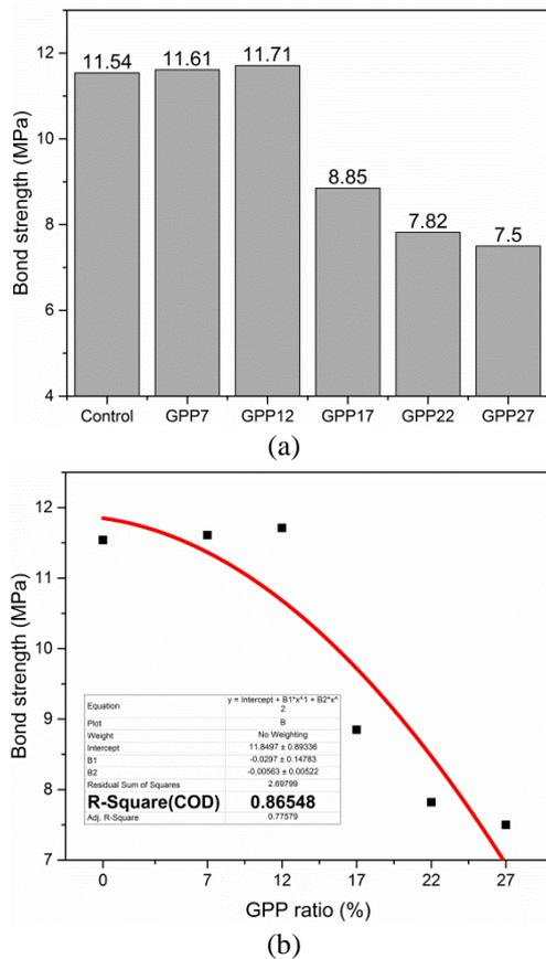
Fig. 11 (a) Bond strength of SCMs of at the age of 28 (b) Variation of bond strengths with respect to GPP replacement at the age of 28 d
