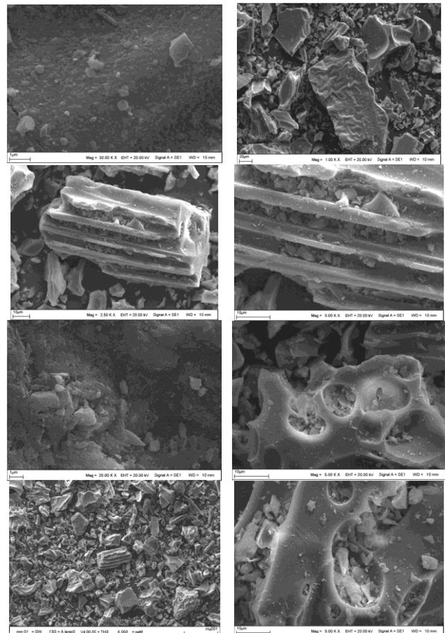
Fig. 7 Microscope images of ground pumice powder
