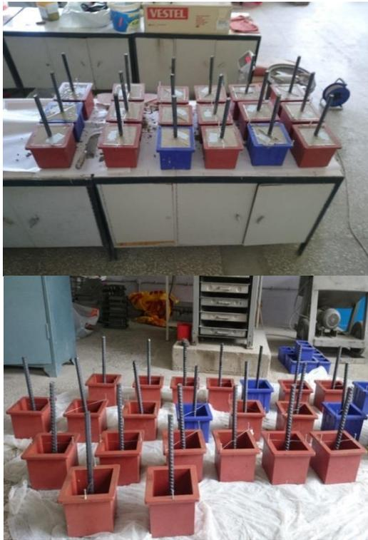
Fig. 1 150×150×150 mm cube specimens for pull out tests
