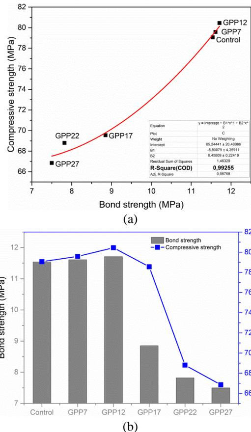
Fig. 12 Variation of bond strengths with respect to compressive strength at the age of 28 d
