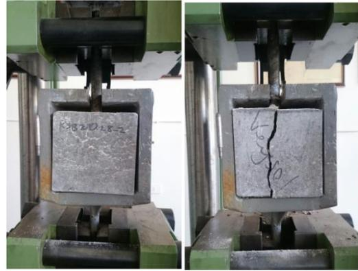
Fig. 4 Pull-out tests of SCMs
