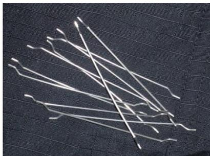
Carbon steel fiber is produced from high-strength cold-drawn steel wire; conform to ASTM 820, widely used for concrete reinforcement
