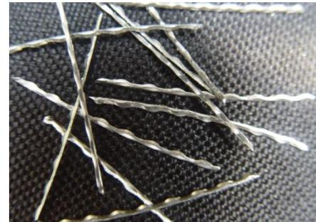
Slit sheet stainless steel fiber is manufactured from coil by chopping the width of the stainless coil, it is used for precast shapes and castable project
