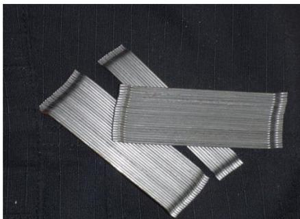
Glued steel fibers are filaments of wire, deformed and cut to lengths, for reinforcement of concrete, with hooked ends. It is easy to separate in the mixer and can avoid balling in concrete matrix
