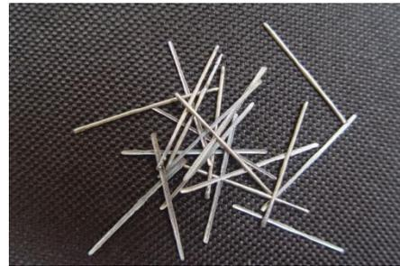
Melt extract stainless steel fiber is produced by melting elements in a crucible. A flywheel is then introduced to the crucible and droplets of molten metal are spun into the open air and hardened
