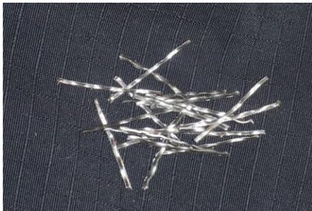
Slit sheet carbon steel fiber is used as a replacement for traditional reinforcement in various concrete applications
