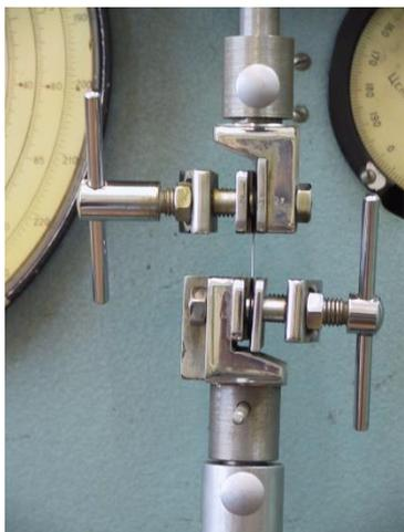
Fig. 3 Steel fibre prepared for tensile strength test
