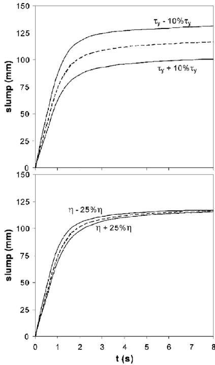
Fig. 9 Simulated slump-versus-time with varying yield stress and plastic viscosity for mix #1
