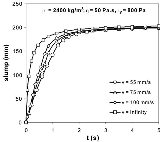
Fig. 20 The effect of withdrawal rate variation on the slump-versus-time spectrum
