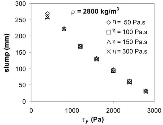
Fig. 17 Yield stress-versus-slump for heavyweight concrete
