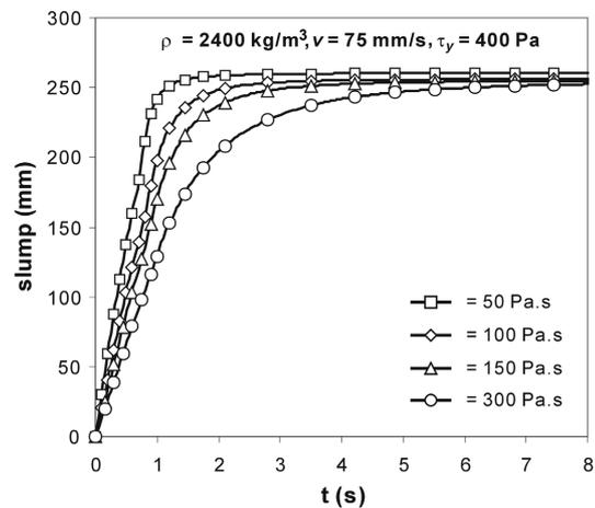
Fig. 19 The effect of plastic viscosity variation on the slump-versus-time spectrum
