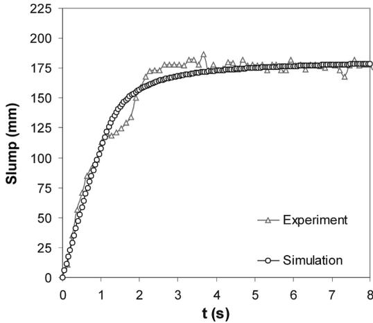
Fig. 6 Recorded and simulated slump-versus-time curve for mix #3
