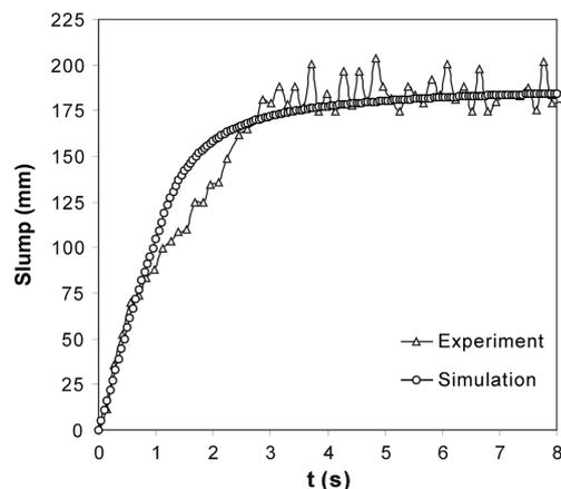
Fig. 5 Recorded and simulated slump-versus-time curve for mix #2
