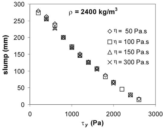
Fig. 16 Yield stress-versus-slump for normal-weight concrete
