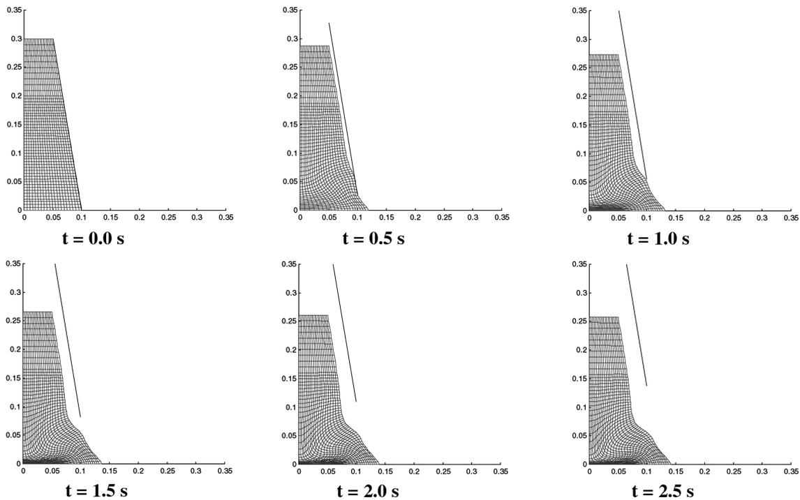
Fig. 2 FE simulation ( $\rho = 2000 \text{ kg/m}^3$ ,  $\tau_y = 1800 \text{ Pa}$ ,  $\eta = 50 \text{ Pa}\cdot\text{s}$  and  $v_{cone} = 55 \text{ mm/s}$ ).
