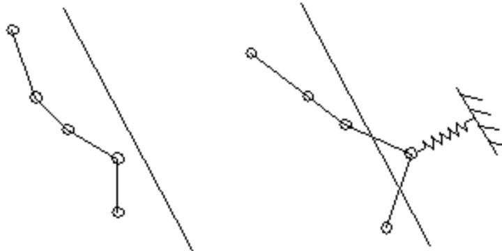
Fig. 1 Schematic view of the spring enforcing contact boundary condition
