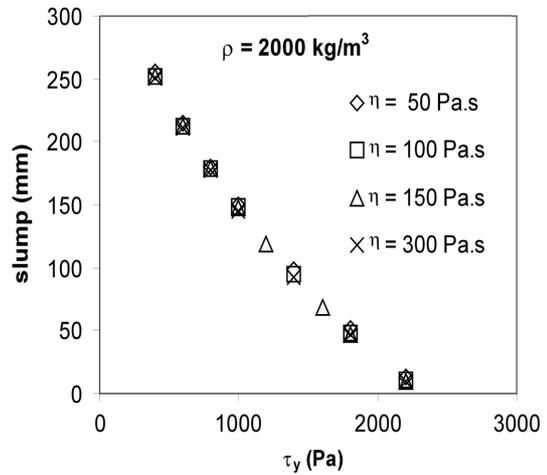
Fig. 15 Yield stress-versus-slump for lightweight concrete
