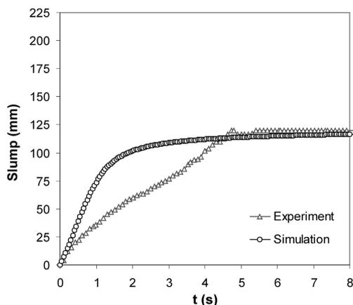
Fig. 4 Recorded and simulated slump-versus-time curve for mix #1
