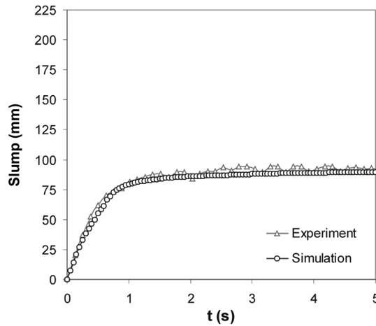
Fig. 8 Recorded and simulated slump-versus-time curve for mix #5
