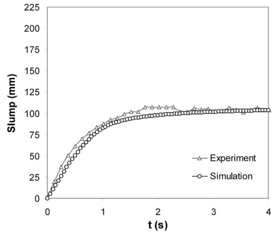
Fig. 7 Recorded and simulated slump-versus-time curve for mix #4
