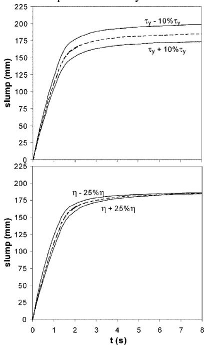
Fig. 11 Simulated slump-versus-time with varying yield stress and plastic viscosity for mix #3
