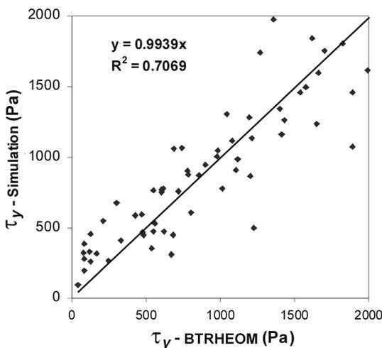
Fig. 18 Comparison between the simulated yield stress and the experimental data
