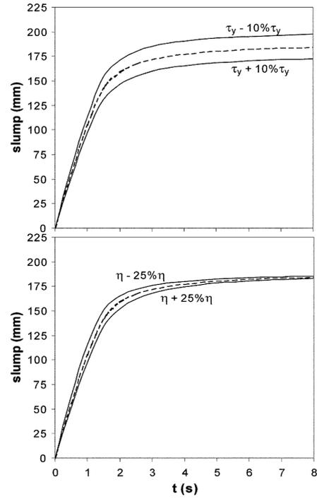
Fig. 10 Simulated slump-versus-time with varying yield stress and plastic viscosity for mix #2
