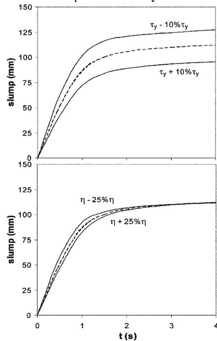
Fig. 12 Simulated slump-versus-time with varying yield stress and plastic viscosity for mix #4
