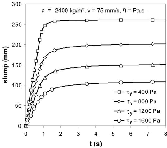
Fig. 14 The effect of yield stress variation on the slump-versus-time spectrum
