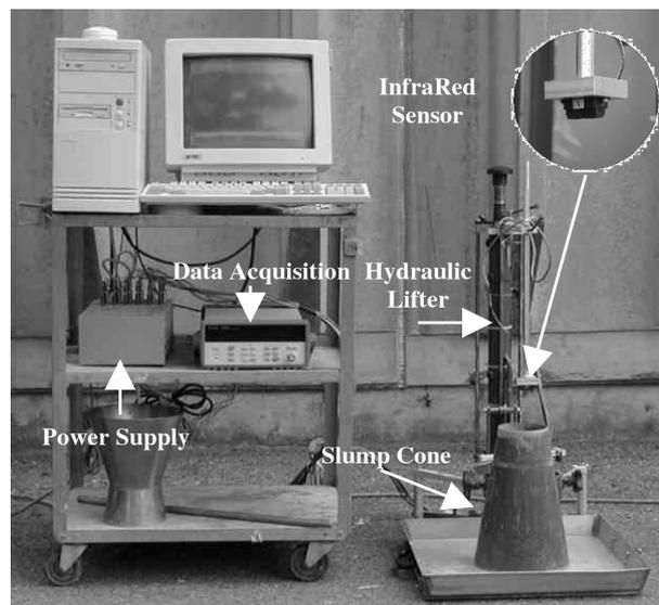
Fig. 3 View of the slump rate machine, SLRM\_II
