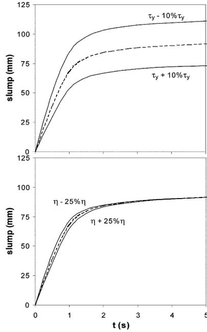
Fig. 13 Simulated slump-versus-time with varying yield stress and plastic viscosity for mix #5
