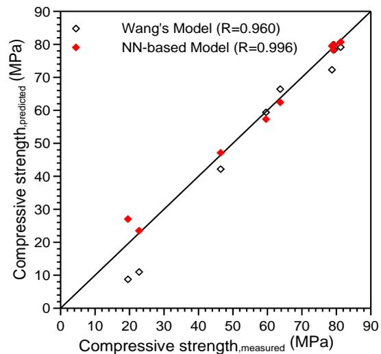
Fig. 8 The comparison of compressive strengths from the algorithms of two predictive models
