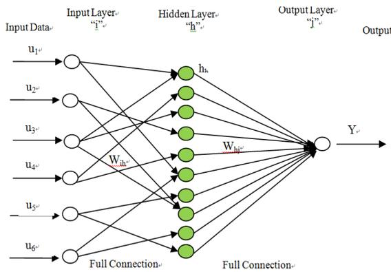
Fig. 1 The network structure of the BPNN
