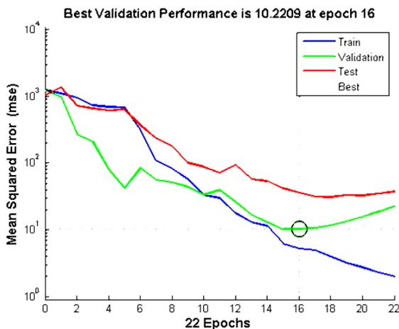
Fig. 7 The learning curve of the NN using the “C” type combination of input variables
