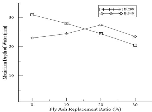
Fig. 9 The maximum depths of water ingress for concretes containing fly ash
