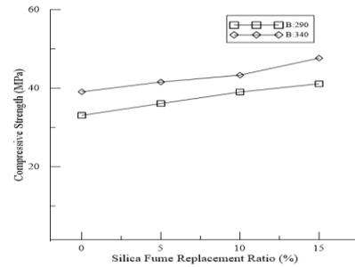
Fig. 14 Compressive strengths of concretes containing silica fume
