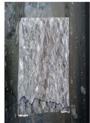
Fig. 4 Marked depth of water ingress
