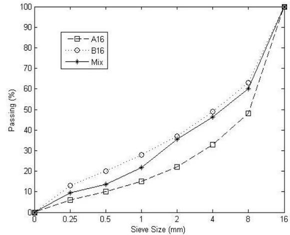
Fig. 1 The gradation of the aggregate mix and the reference curves
