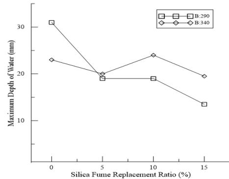
Fig. 10 The maximum depths of water ingress for concretes containing silica fume
