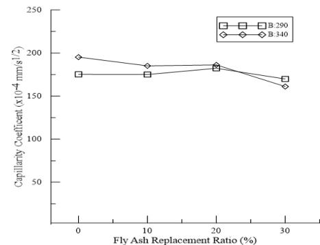
Fig. 11 Capillarity coefficients for concretes containing fly ash
