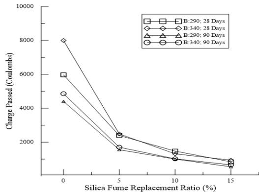
Fig. 8 Rapid chloride permeability for concretes containing silica fume
