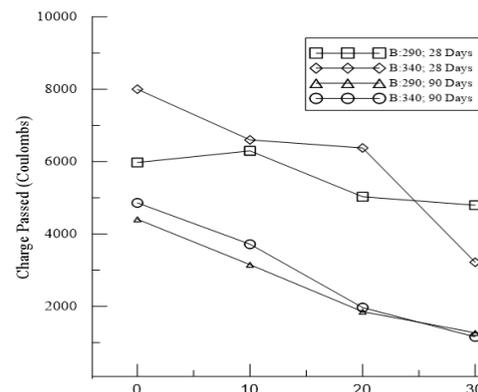
Fig. 7 Rapid chloride permeability for concretes containing fly ash
