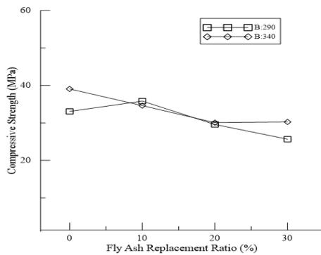
Fig. 13 Compressive strengths of concretes containing fly ash
