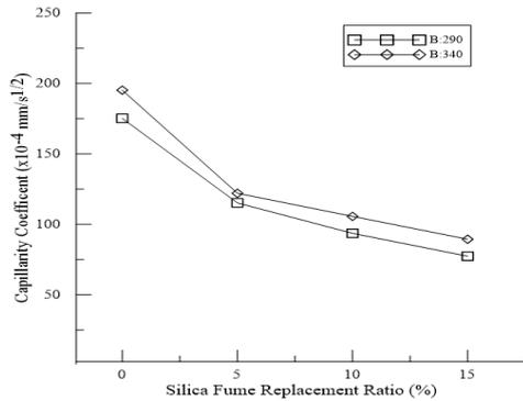
Fig. 12 Capillarity coefficients for concretes containing silica fume
