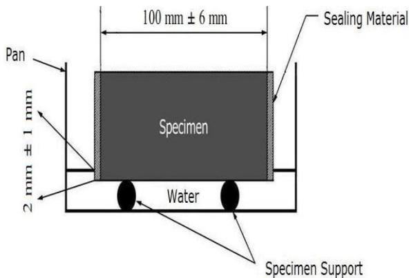
Fig. 5 Set up for the capillary test (ASTM C1585)
