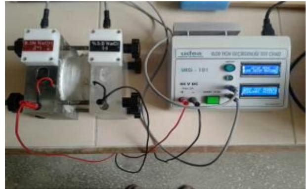
Fig. 2 Set up for rapid chloride permeability test
