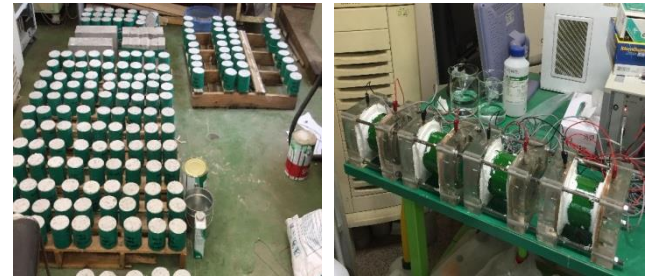
Fig. 4 Photos for test setup of diffusion cell in steady state condition
