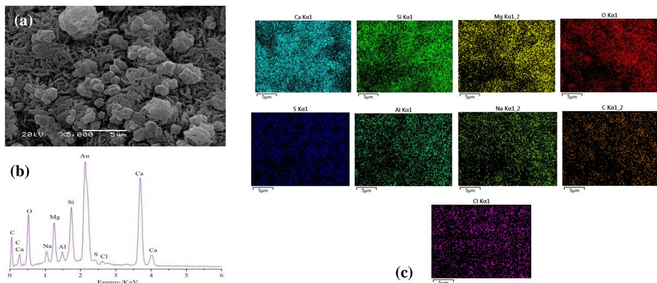
Fig. 4 SEM images of microstructures and plan scanning analysis of sample from ACC2: (a) surface morphology, (b) result of plane scanning, (c) elemental mapping on the sample surface of Ca, Si, Mg, O, S, Al, Na, C, Cl
