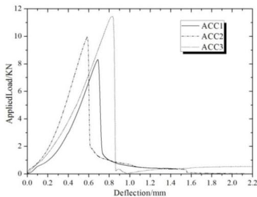
Fig. 2 Load-deflection curves of different specimens
