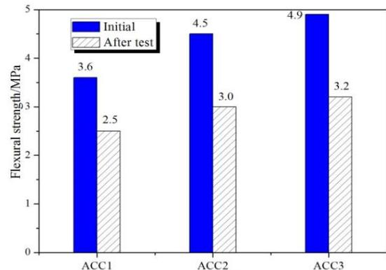
Fig. 3 The flexural strength of different group specimens
