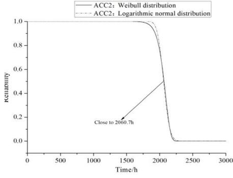
Fig. 5 The reliability curve of different methods
