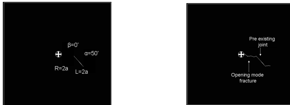
Fig. 9 The opening mode fracture initiation for L=2a
