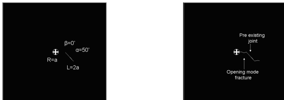
Fig. 11 The opening mode fracture initiation for joint offset angles of 50^\circ .
