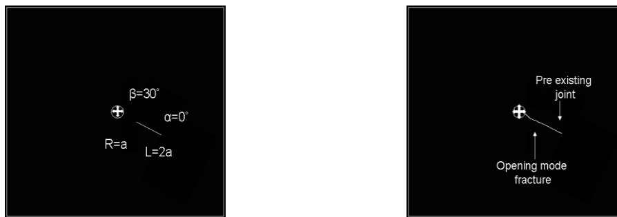
Fig. 13 The opening mode fracture initiation for two joint length; L=2a
