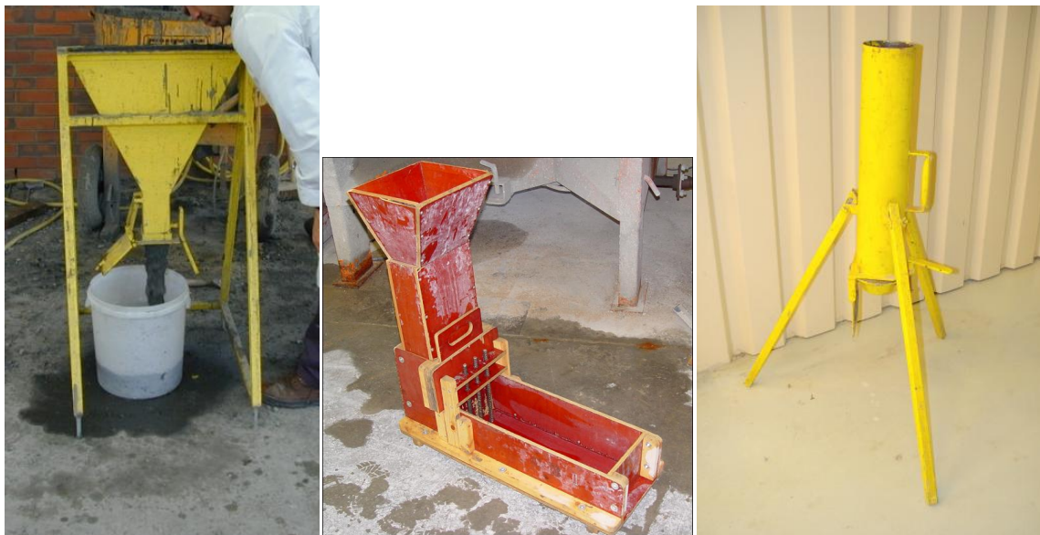
Fig. 2 V-funnel, L-box, and Orimet tests
