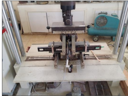
Fig. 2 Beam under loading to do flexural toughness test
