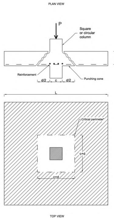
Fig. 2 Typical geometry configuration of FRP-reinforced two-way slabs
